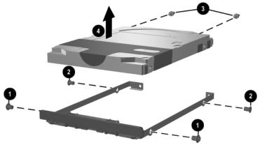
Removing the Hard Drive from the Hard Drive Frame
